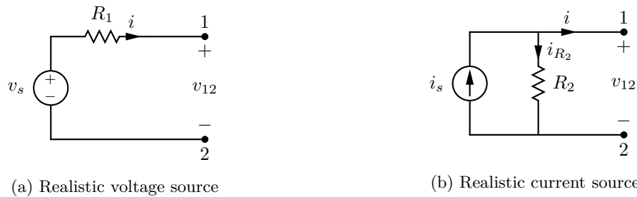
Figure 15: For a certain choice of R_1 = R_2 and i_s = \frac{v_s}{R_1} these are equivalent
